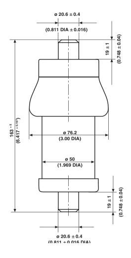
Noble metal electrodes completely lacquered. Insulating rim glazed.
